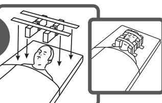
**ENG** All elements of the head blocks can easily be adjusted with the hook and loop fasteners. Position two elements of the head blocks next to head. Place them above each other. Do this on both sides. Head and chin straps hold the head securely in place.
